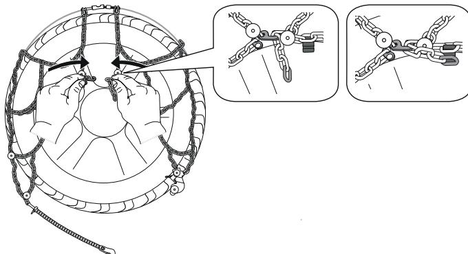
**EN** Each snow chain can fit several tyre sizes. It may happen that an adjustment of the snow chain dimension might be required in order to perfectly fit the tyre. This adjustment can be done using the adjusting links on the upper side chain.
